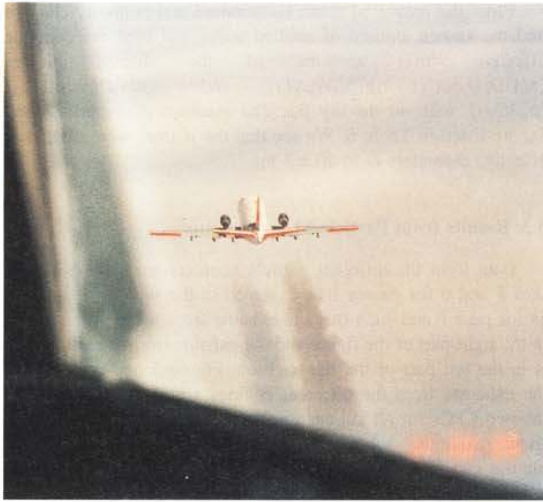
Plate 2. Photo of the ATTAS flying with different fuels as seen from the Falcon cockpit at a distance of about 150 m, at 1100:25 UTC, at FL 307 (9360 m) on a course toward NNE.
