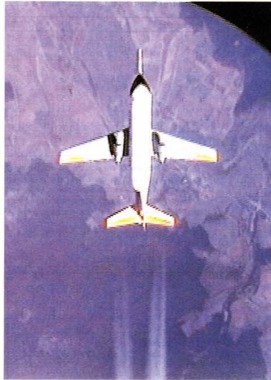
Plate 1. Printed video scene with view from the Falcon 150 m above the ATTAS aircraft at 1055 UTC, 49°50'N, 11°30'E, ATTAS at FL 310 (9450 m), burning fuels with different sulfur contents (170 ppm left, 5500 ppm right).
