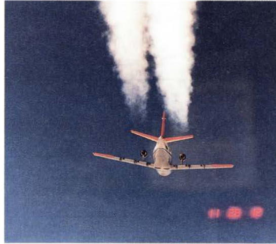
Plate 3. Photo of the ATTAS flying with different fuels as seen from the Falcon cockpit at a distance of less than 100 m, at 1128:12 UTC, at FL 300 (9140 m) on a course toward SWS.
