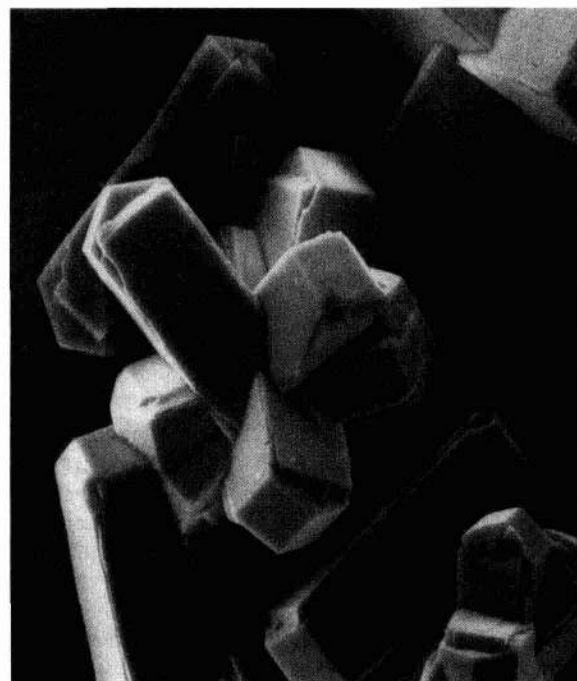
Figure 5. Scanning electron microscopy (SEM) picture of some crystals of zeolite ZSM-5, a catalyst material for methanol-to-olefins (MTO) conversion.
