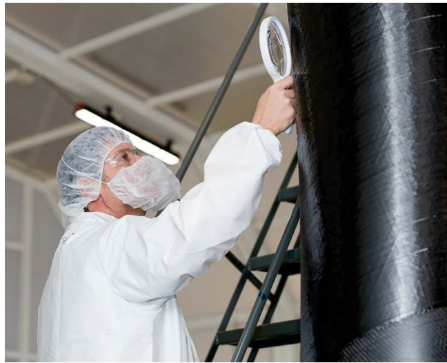
FIGURE 2. Example of actual visual inspection of a composite AFP part.
