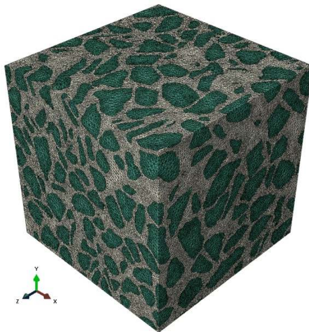
Fig. 14 The modelled RVEs (10mm, 20mm, 30mm and 37mm): aggregates in yellow, cement in green and voids in blue; not up to scale
