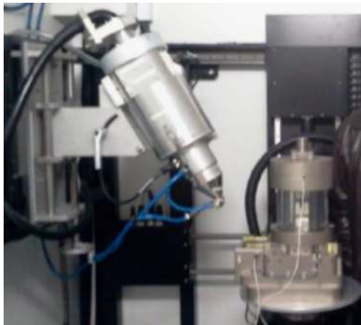
(a): The in-situ XCT facility in MXIF
