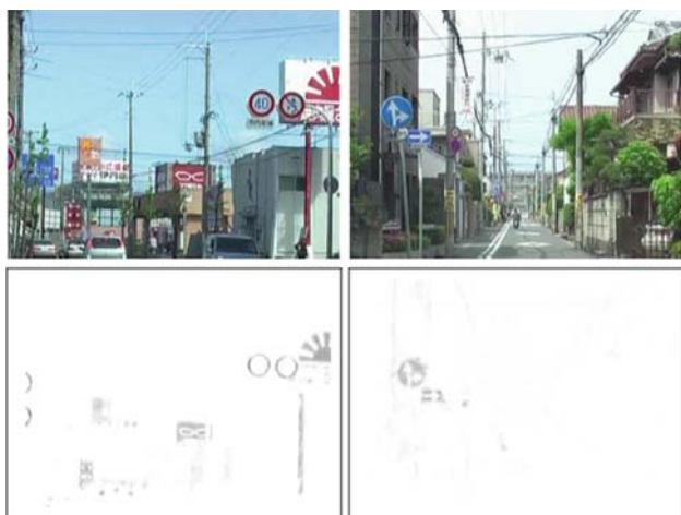
Fig. 2 The effect of applying the color filters (3) to the example RGB images (top row): red color filter (bottom-left), blue color filter (bottom-right)
