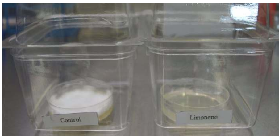
Fig. 1. Effect of limonene on the growth of T. rubrum in vapor contact assay. Control Phytatray (left) shows fungal growth. Limonene treated Phytatray (right) shows no fungal growth.
