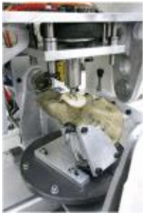
The Portsmouth four station hip simulator with a specimen loaded in one of the test cells
