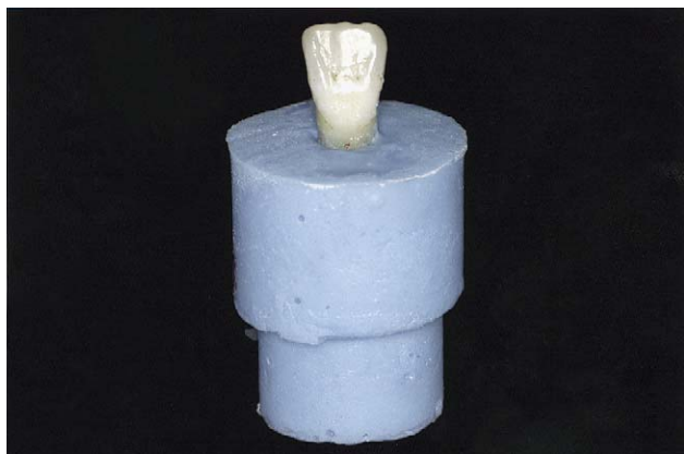
Fig. 2. Specimen mounted in acrylic block.
