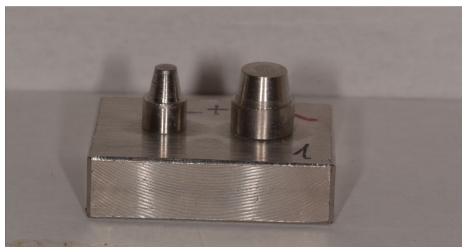
Figure 1. Three-units master abutments
