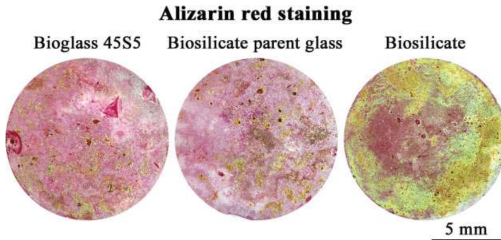
Figure 5. Macroscopic images of osteogenic cultures grown on Biosilicate ® glass-ceramic, on control bioactive glasses Bioglass ® 45S5, and Biosilicate ® parent glass, stained with Alizarin red at day 17. Biosilicate ® supports larger amounts of bone-like matrix formation (yellowish areas in a reddish background). [Color figure can be viewed in the online issue, which is available at www.interscience.wiley.com .]
