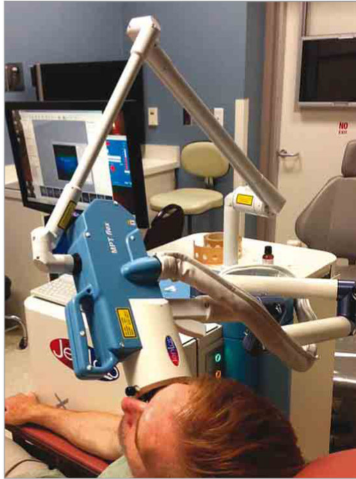
Figure 1. The Imaging Procedure of a Skin Lesion on the Face Using the multiphoton microscopy (MPM)-based clinical tomograph (MPTflex).
