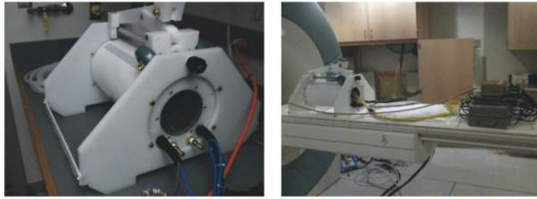
FIG. 1. The actively-shielded, liquid-cooled Z_2 insert coil on the test bench (left) and mounted on the patient table with accompanying RF hardware.
