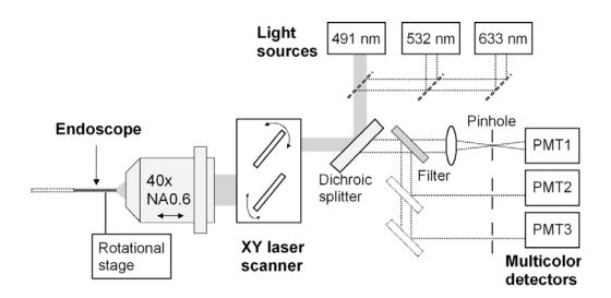
**Supplementary Figure 1**: Schematic of the imaging system. The imaging head is reconfigurable to mount the objective lens and endoscope vertically.
