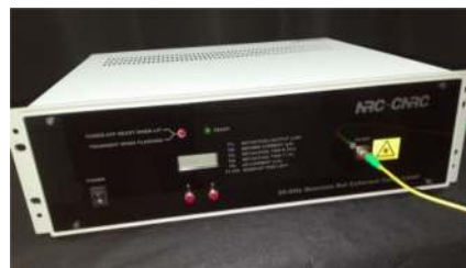
Fig. 8. A completed rack mount QD C-band 25 GHz CCL module.
