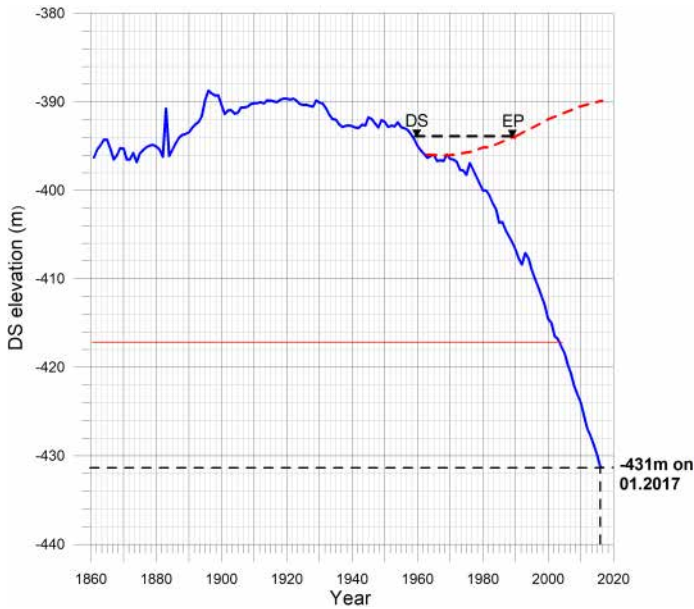
Fig. 2. Variations of the DS level during last 157 years. Thick solid line, DS (northern basin); red dashed line and EP (evaporation ponds, southern basin); red thin line – salt top elevation at the Nahal Hever South (NHS) site (data of the Geological Survey of Israel).
