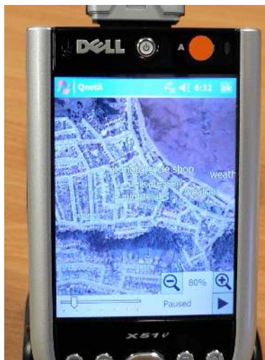
Figure 1. Prototype runs on a PDA device with GPS for location information.
