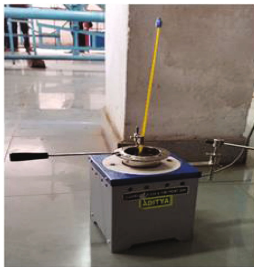
FIGURE 3: Cleveland flashpoint and fire point apparatus.
