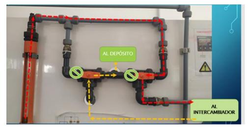
**Figure 2.** Capture from the concentric tubes heat exchanger AR-based Project. Dark green box text: "To the tank" in Spanish. Light green box text: "To the heat exchanger" in Spanish.
