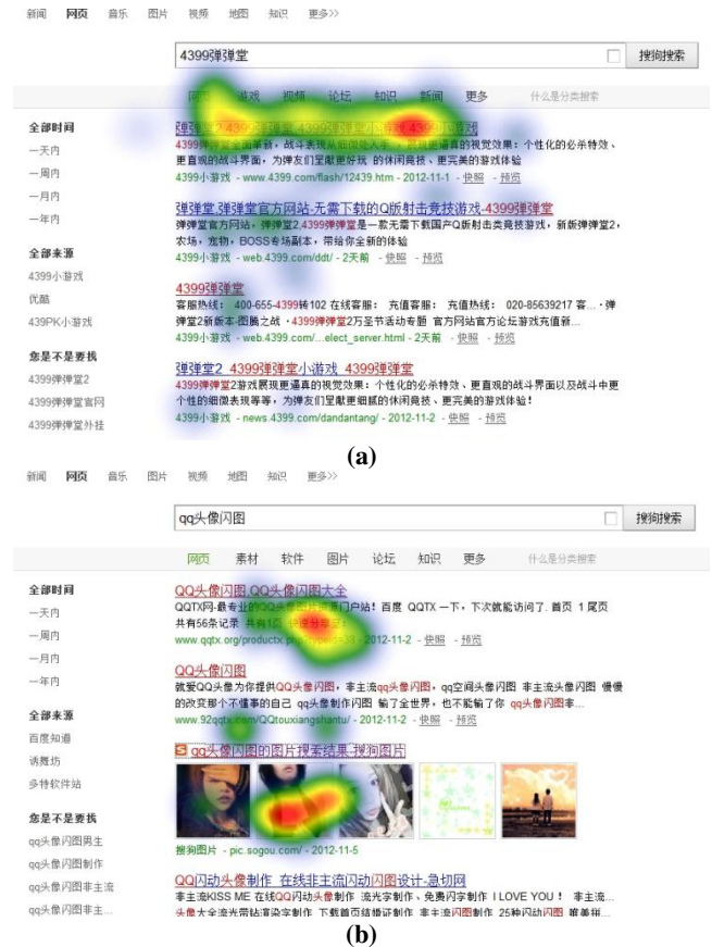
Figure 8. Heat map of the subjects' eye fixation areas in first 2 seconds on (a) SERP with no vertical (b) SERP with multimedia vertical placed at the 3 rd position
