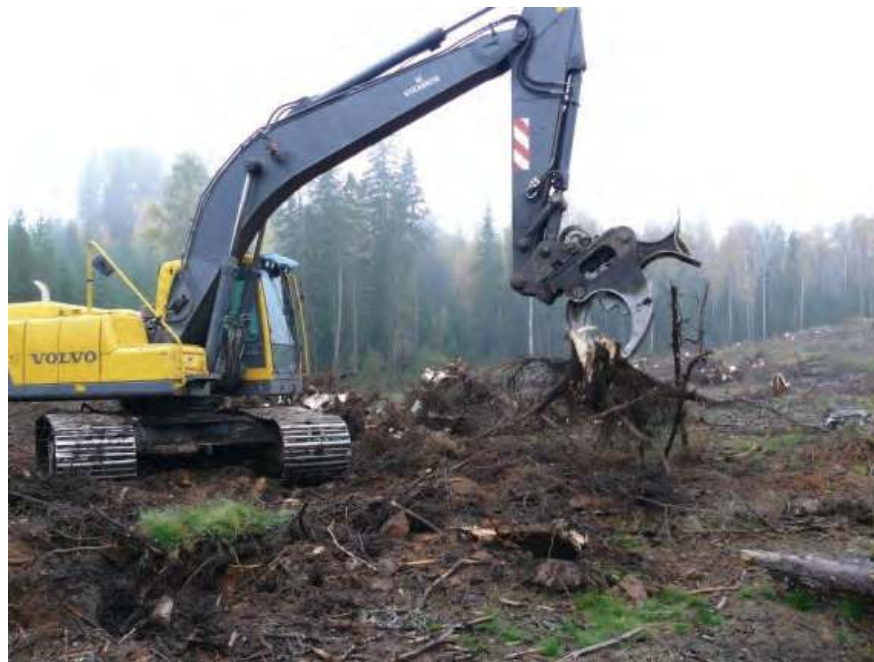
Figure 3 Current stump-harvesting technique; an excavator with a stump-lifting head is used to lift the stumps and cut them into pieces. Photo: Pär Aronsson.
