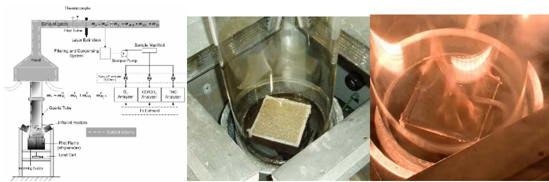
Figure 5.2 a) Schematic of the Fire Propagation Apparatus (FPA)
