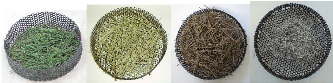
Figure 2.2 Pinus halepensis needles samples for a) Live b) Aged c) Dead d) Ash after burn
