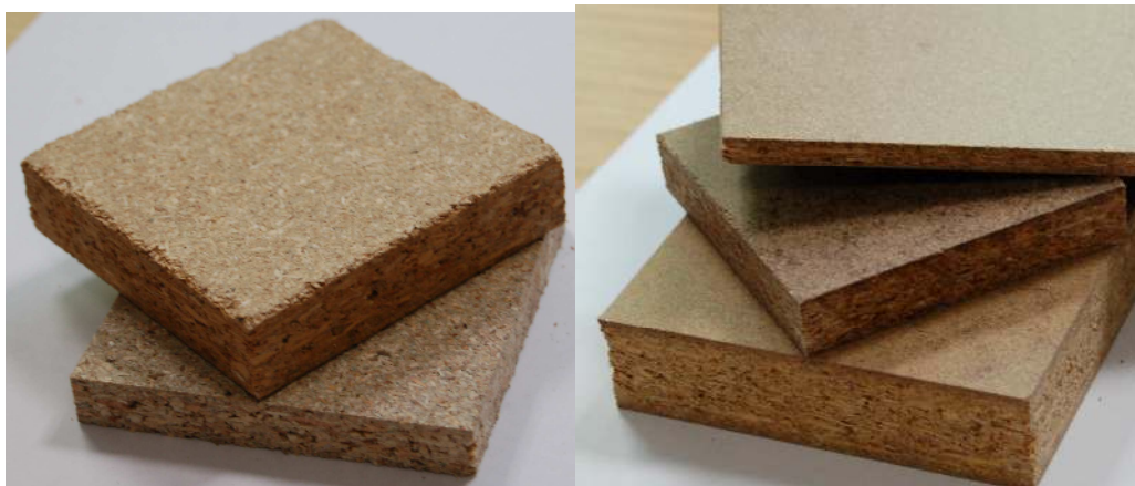
Figure 5.1 a) 12 and 18 mm thick Chipboard LD b) 6, 15, and 25 mm thick Chipboard MD
