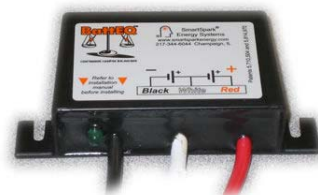
Fig. 5. Equalizer for two 12V lead acid batteries rated up to 50 A-hr
