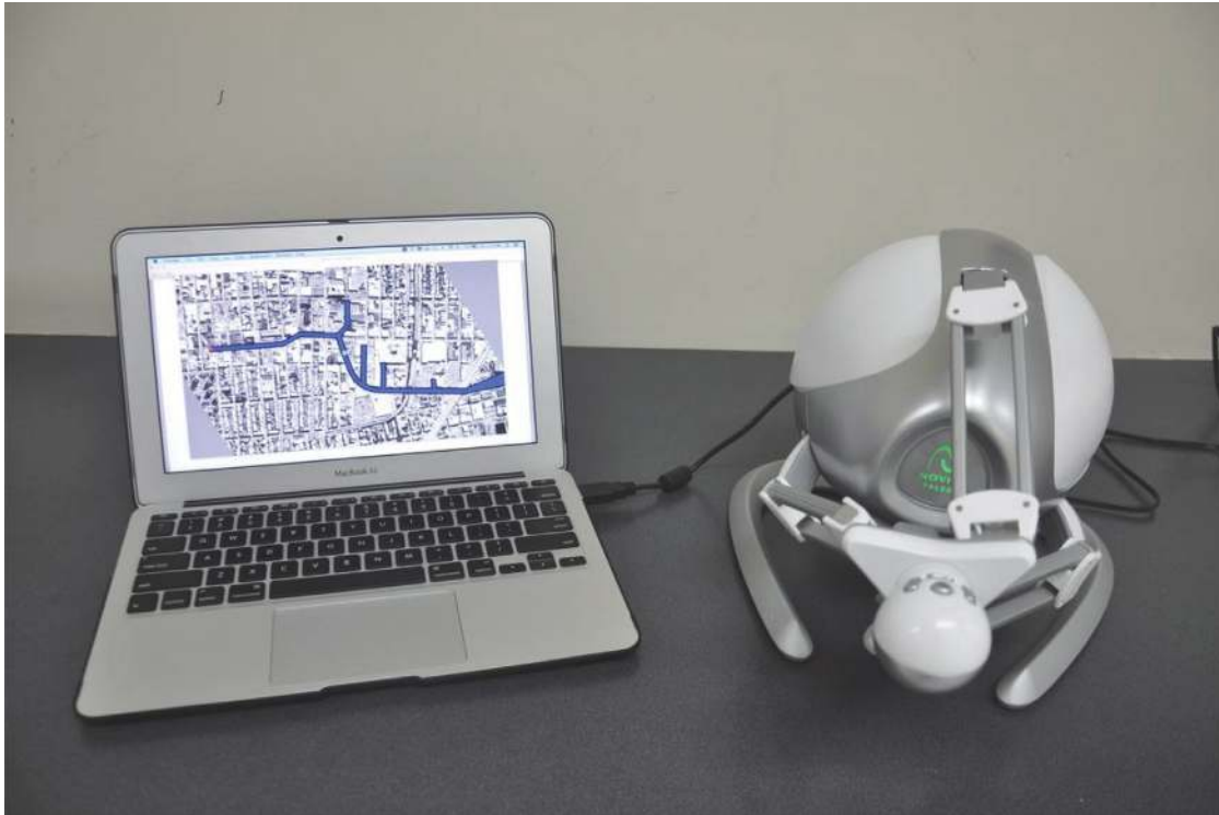
Fig 1. The experimental setup, consisting of a laptop computer and a Novint Falcon haptic device.
