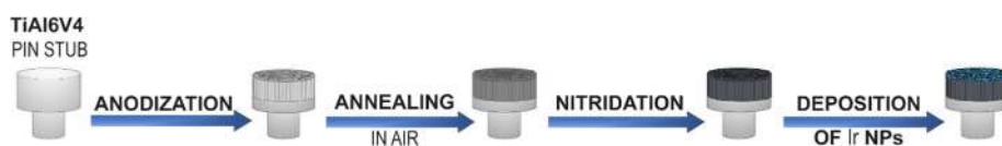
Figure 1. Procedure for preparing the immobilized TiON–Ir thin-film electrode.
