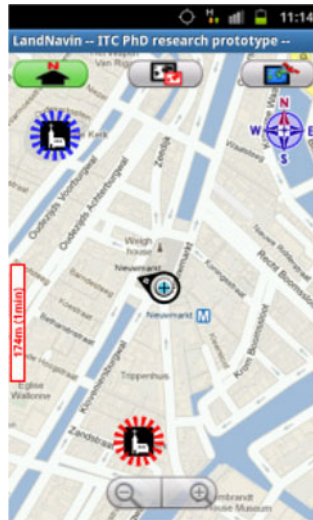
Figure 6. LN interface showing two global landmarks (churches). One is visible (blue dashed circle around landmark symbol) and the other is invisible (red dashed circle around landmark symbol) from the current position.
