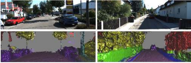
Fig. 5: Our approach not only reconstructs and labels entire outdoor scenes that include roads, pavements and buildings, but also accurately recovers thin objects such as lamp posts and trees. See Fig. 1 for colour coding.
