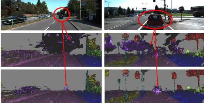
Fig. 6: Our semantic fusion technique enables us to avoid corrupting a static scene with data from moving objects. First row: input image; second row: reconstructed scene without semantic fusion; third row: reconstructed scene with semantic fusion. Note the way in which semantic fusion helps suppress the trail of spurious voxels that moving objects would normally leave behind. See Fig. 1 for colour coding.
