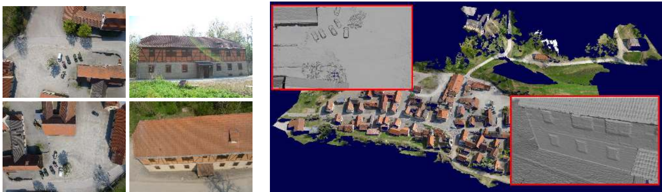
Figure 7. On the left four example images of a registered image set of 822 images are shown. The right part presents a screenshot of the colored surface model reconstructed by [15] from 1.5 billion points and shaded zoomed parts from the surface model demonstrating the preservation of small details. In spite of the space division, the 3D model has consistent surfaces.
