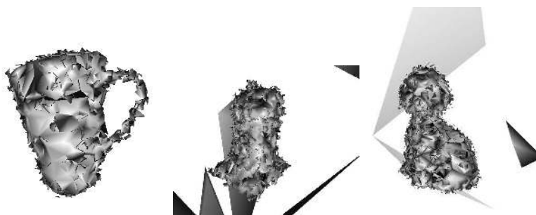
Figure 5.9: Noisy reconstructions. The point-cloud sampling standard deviation is 2% of the bounding box scale, with a 1% outlier rate. Sampling was dense. From left to right: Cup, House2, Dog.
