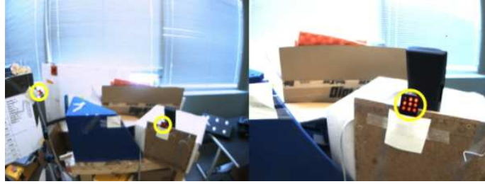
Figure 5.18: An operator performing inspection. Left: Target locations are seen from far away. Right: But identification of the burnt LED requires a close view.
