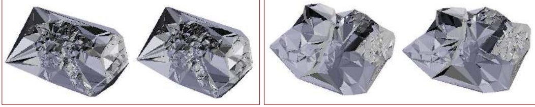
Figure 5.4: Results for K = \infty (left) and K = 1 (right) on different data sets. The meshes are similar for extremely different K .
