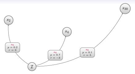
Expansion function  $\mathcal{S} \times \mathcal{A} \to \mathcal{P}_r(2^{\mathcal{S} \times \mathbb{R}})$  indicating all probabilistic successor states and rewards from a state and applying a given action
