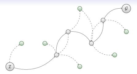
Select and expand tip-nodes by considering all probabilistic effects of each state in the graph  $\Rightarrow$  new tip-nodes
