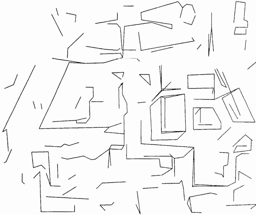
FIG. 17. Result of pruning the junction connections in Fig. 15 by determining whether segments in Fig. 13 adequately cover the area between each pair of connected junctions.
