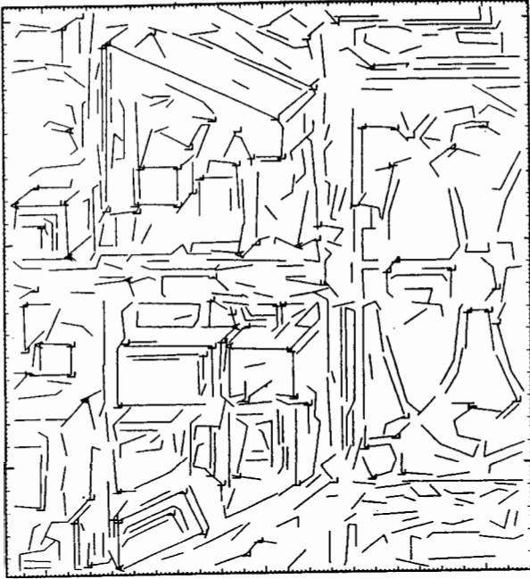
Fig. 5. Result of classifying junctions extracted from the images in Fig. 4. Junctions are classified as L, A (arrow), F (fork), or T.
