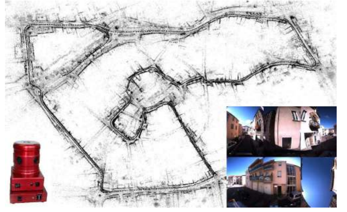
Fig. 5. Global overview of the SfM points cloud of our test trajectory as well as an example of the Ladybug camera image.
