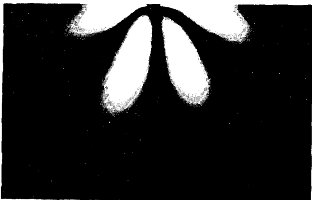
Figure 14—Line flaw in soda-lime glass, produced by tungsten carbide glass-cutting wheel. End view, in polarized light, showing residual stresses about track. After reference [48].
