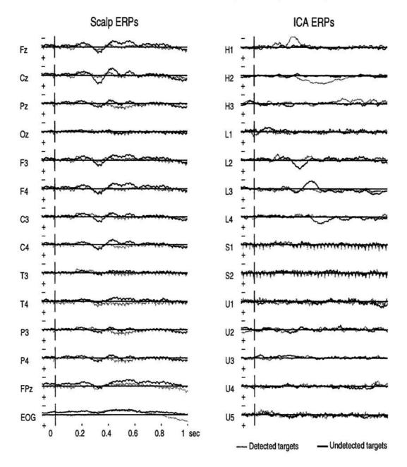
Figure 2: Left panel: Event-related potentials (ERPs) in response to undetected (bold traces) and detected (faint traces) noise targets during two half-hour sessions. Right panel: Same ERP signals filtered using an ICA weight matrix trained on the ERP data.
