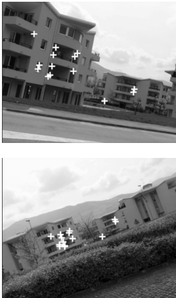
Figure 7: Example of images taken from different view points. There are 14 inliers to a robustly estimated fundamental matrix, all of them are correct. The estimated scale factor is 2.7.
