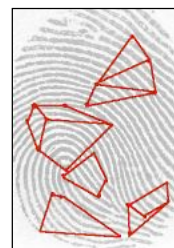
Figure 1: Sample minutiae quadruplets in a fingerprint image.
