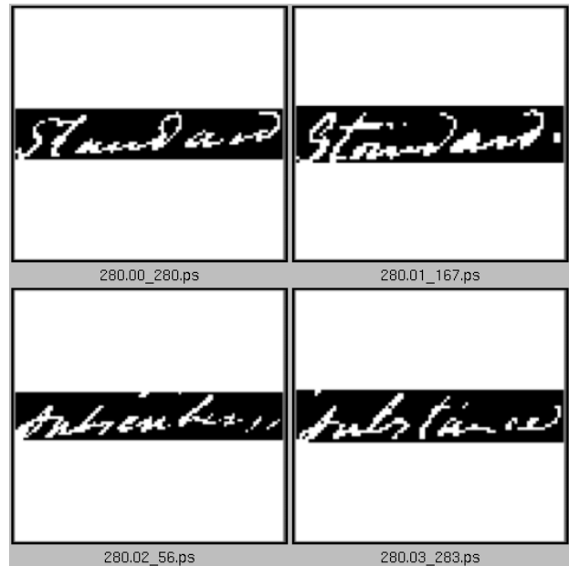
Figure 10: Rankings for template “Standard” using an affine matching algorithm (the rankings are ordered from left to right and from top to bottom).
