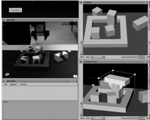
Figure 20: Screen image at operator site. Left window: Camera image window. Upper right window: Feedback model window, showing the latest model of the remote site, as given by the vision module. Lower right window: Object manipulation window. This is periodically initialized to the state of the feedback model window, but then is changed according to operator interactions.
