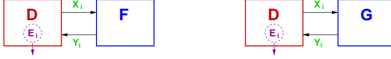
Fig. 5. Distinguishing two (\mathcal{X}, \mathcal{Y}) -random systems \mathbf{F} and \mathbf{G} by means of a distinguisher \mathbf{D} . The figure shows the two random experiments under consideration.
