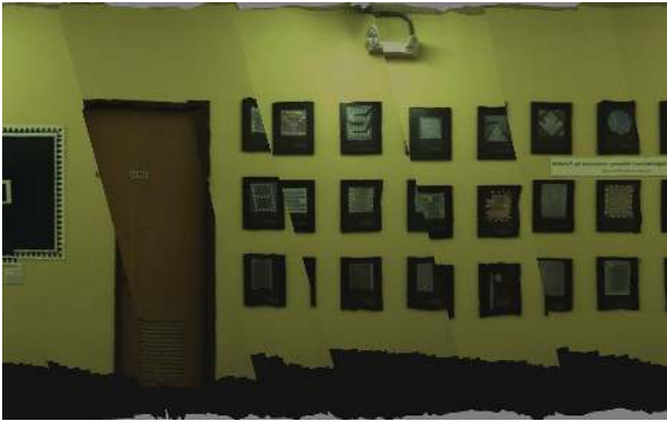
Fig. 10. Screenshot of textured 3D model generated from localization data without image based refinement. Misalignments between textures from different images are apparent.
