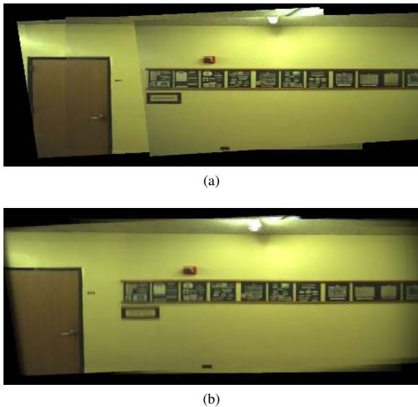
Fig. 15. The results of mosaicing images together (a) before and (b) after alpha blending. Note the elimination of the boundary artifacts.
