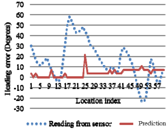
Figure 6. The blue graph plots raw heading directions directly extracted from the sensor reading. The red graph shows the heading directions predicted by the system. The x-axis represents locations along the corridor and the y-axis represents the heading error in terms of degree.
