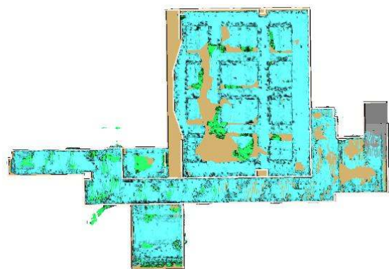
Figure 9. Hololens mesh (in cyan colour) registered with the reference 3D model.
