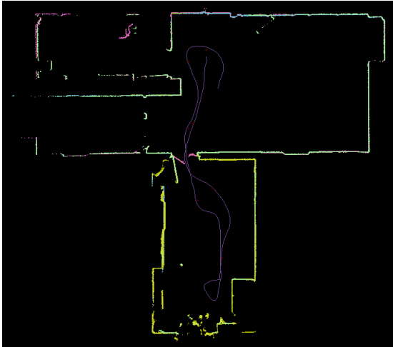
Figure 9. iMMS processed SLAM solution trajectory loop of office in Viametris PPIMMS software
