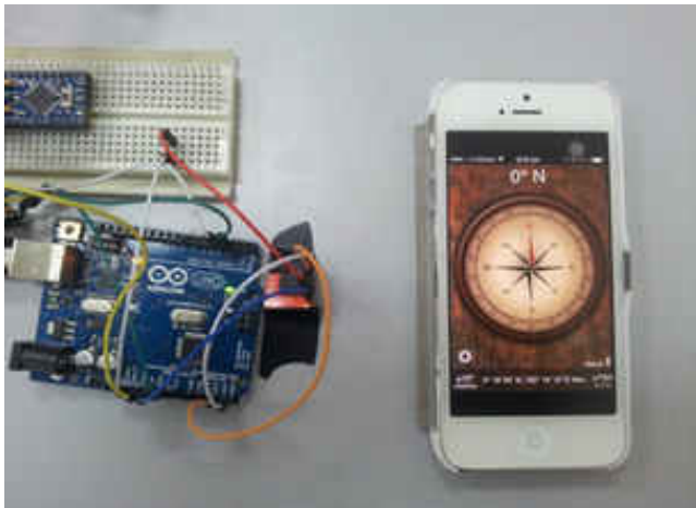
Fig. 7. Digital compass setup and the reference compass
