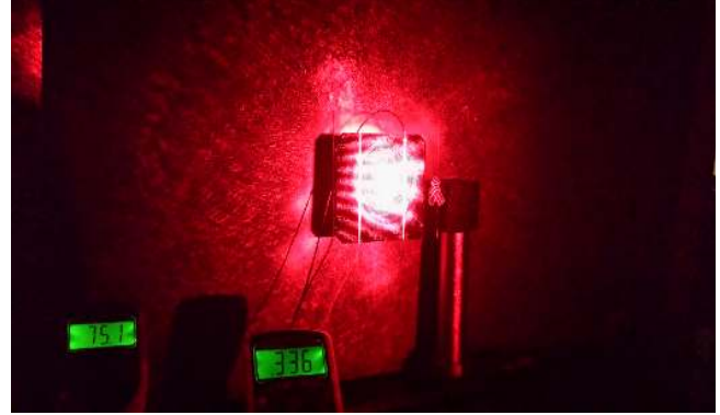
Fig. 5. Scenario II: Beam pattern of three laser sources and measurement of P_m .
