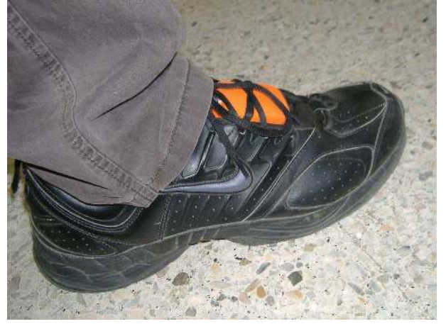
Fig. 6. Xsens IMU attached to the right foot using the shoe's laces.
