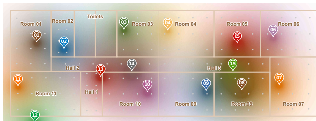
FIGURE 4. Signal characterization of the environment using the signal propagation model as executed by the RSSI simulator.
