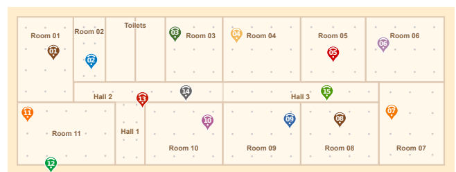
FIGURE 3. Real-world experimentation testbed: 11 rooms, 3 halls, and 15 anchor nodes. Gray dots represent the 150 reference points.
