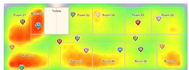
FIGURE 15. Heat-map of the average errors for all test points in the scenario.
