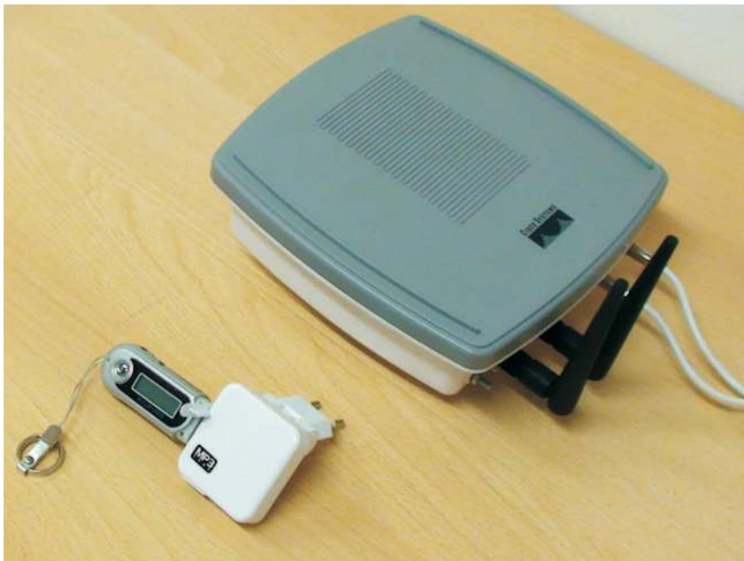
Figure 4.2: FM transmitter and Wi-Fi access point.
