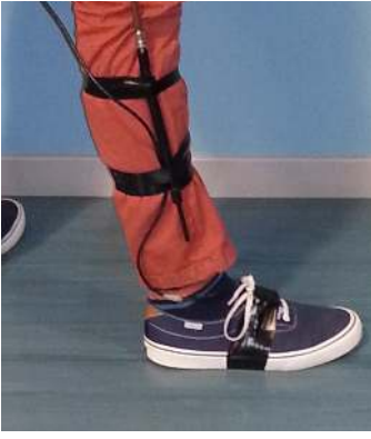
Fig. 1. Foot-mounted INS and antenna mounted on right leg of a user about to perform one of the experiments.
