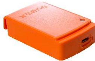
Fig. 4. An IMU containing a 3-axis accelerometer and a 3-axis gyroscope.
