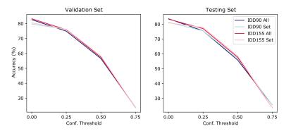
**Figure 2.** Scene Recognition for IOD90 & IOD155—visualization of results across conf. thresholds (0.001, 0.25, 0.50, 0.75) for validation and testing sets. Also displayed are whether all detected objects or singular instances (sets of objects) are used in predicting room category.
