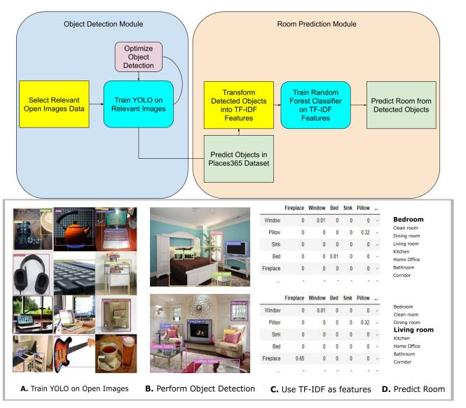
**Figure 1.** Visualization of the pipeline. *top*: general diagram of the modules for object detection and room prediction, and *bottom*: step-by-step scheme (**A**) Train YOLO to detect indoor objects. (**B**) Perform object detection on scene data (examples use IOD155 with conf. thresh = 0.25). The images are from the ADE20k dataset (**C**) Transform predicted object labels into TF-IDF input features. (**D**) Train classifier to predict room category based on these input features.
